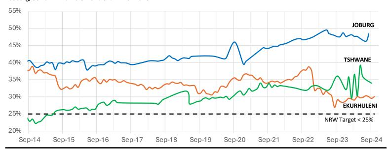
**8. REAL OR PHYSICAL LOSSES 10-year TREND:** This is the volume of water that runs to waste without any user using it. This includes leaks on mains, leaks and overflows on storage infrastructure and on service connections *outside private property boundaries*. While NRW management includes financial losses, Real losses impact directly on the volume of water that is used. The target is < 15%, shown below.
